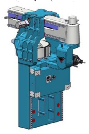
Main Milling Unit: 8.7 kW (max), 20.000 R.P.M HSD motor Machining accuracy (X,Y,Z) : +/- 0.05 mm
