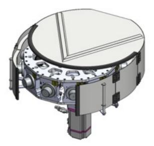
• Noise isolation cabinet around the machining head
