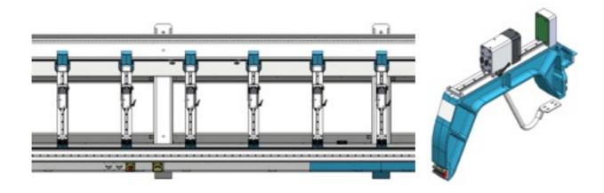
• 2 pieces of pneumatically operated supports to determine the reference of workpiece in X- direction
