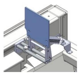
• Saw magazine up to Ø180 of saw blade
