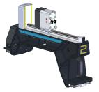
• 2 pieces of pneumatically operated supports to determine the reference of workpiece in X- direction
