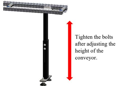
Tighten the bolts after adjusting the height of the conveyor.
